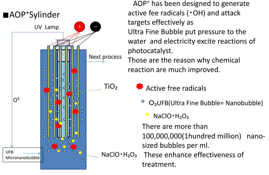
NaClO and  $H_2O_2$  are used for the purpose of promoting reaction in AOP. They might not be used depends on conditions of waste water as we usually decide it according to the result of pre test.
